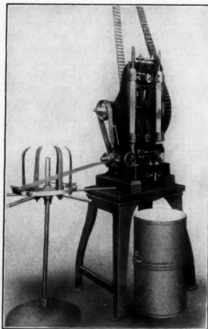
FIG. 6 — SPECIAL MACHINE FOR BLANKING, PIERCING AND FOLDING BOW LINKS
